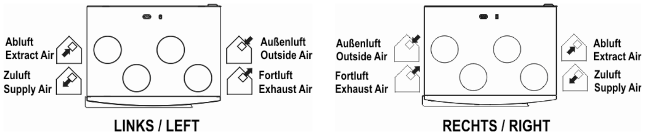
Figure 22: Tag of the connection of the air ducts
