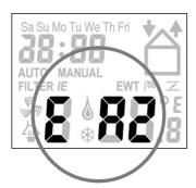
A flashing "Filter I" or "Filter E" below the field displaying the ventilation modes.
