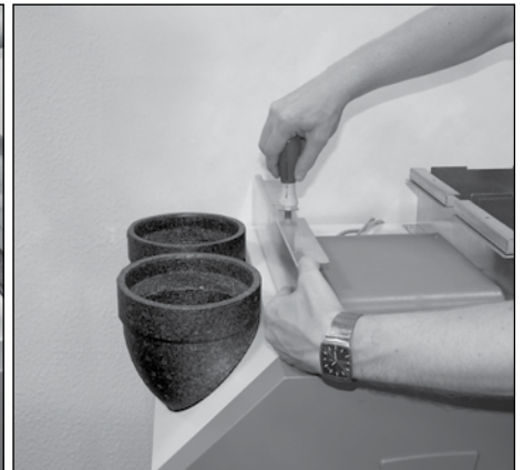
3. Locate U-profile and screw onto the CA 350
