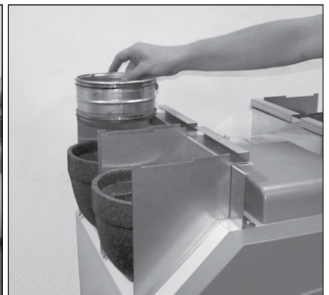
6. Insert the 160 mm nipple into the CA 350
