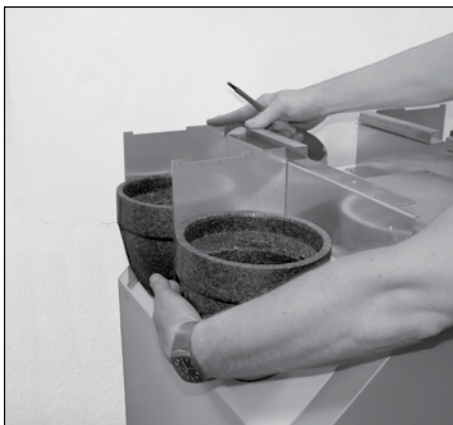
4. Attach the mountings to the U-profile
