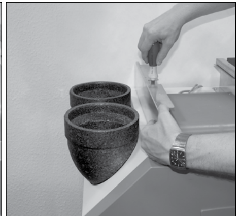
3. Locate U-profile and screw onto the CA 350
