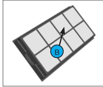
5. Slide the new filters back into the ComfoAir.
