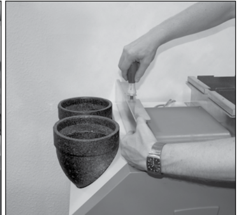
3. Locate U-profile and screw onto the CA 350
