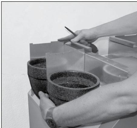
4. Attach the mounting to the U-profile
